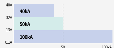
MMS-32H MMS-32HI • High break • Magnetic release
