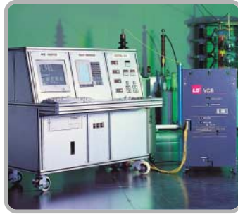
Characteristics Test / VCB Characteristics Test
